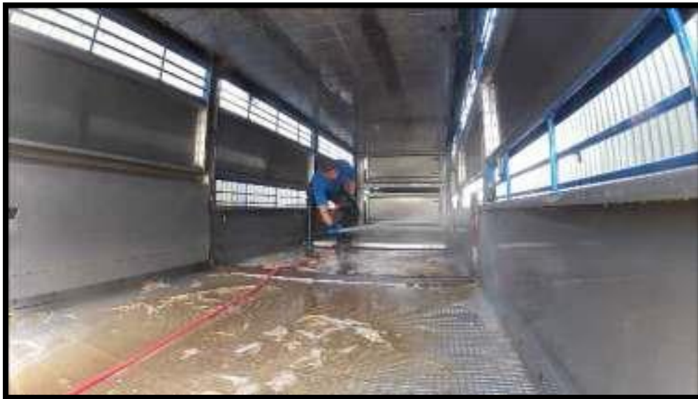
Operator removes all visible soiling with a clean pressurised water wash.
